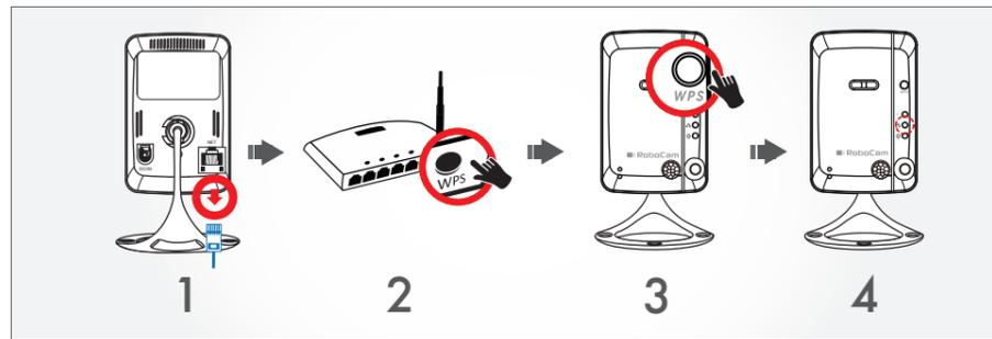
1. Remove the Ethernet cable from the camera.
