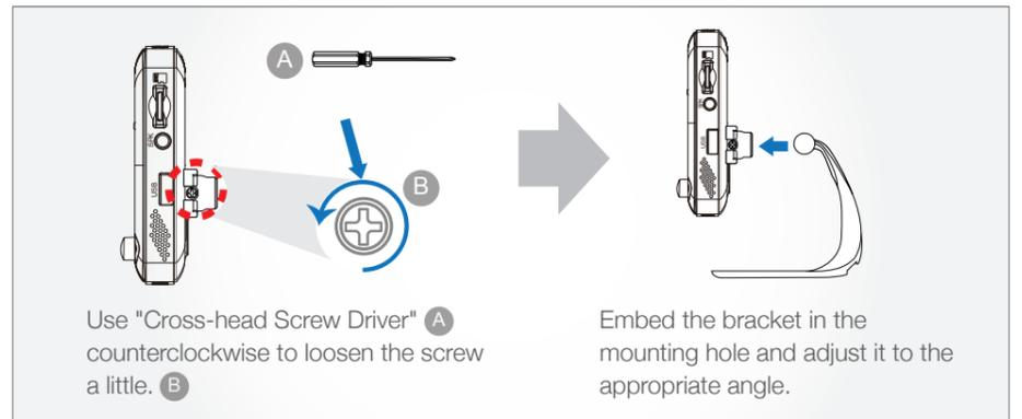
Embed the bracket in the mounting hole and adjust it to the appropriate angle.
